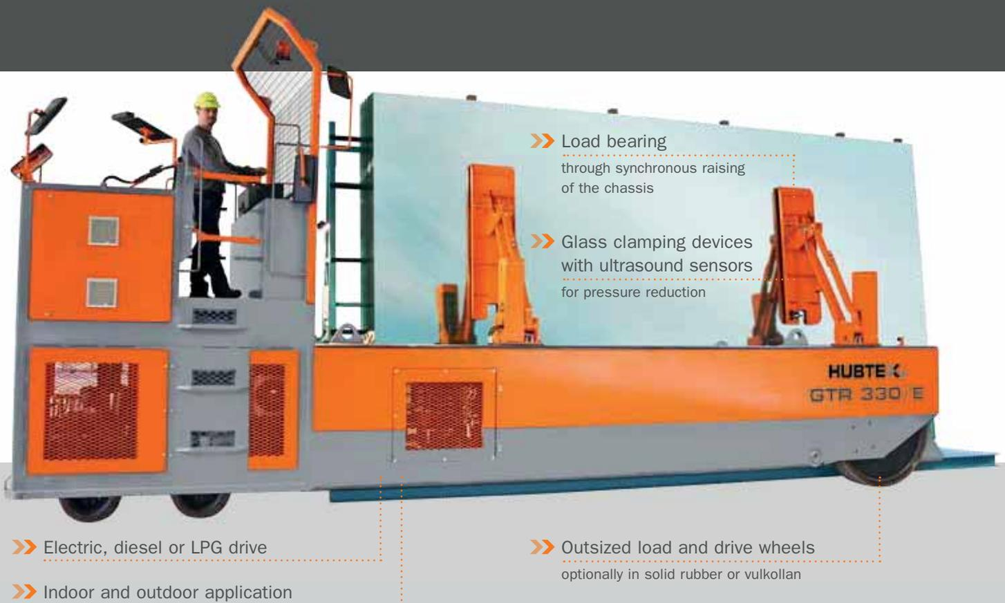
» Load bearing through synchronous raising of the chassis
