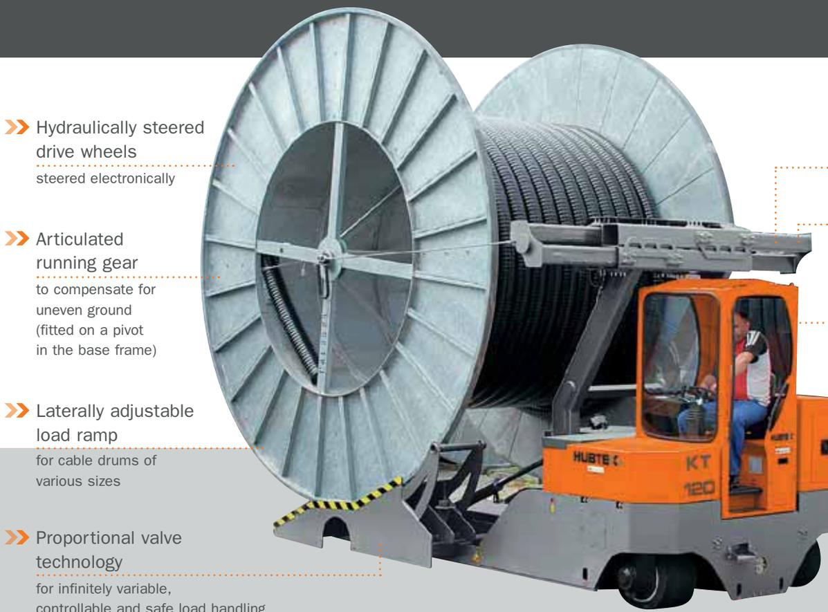
Hydraulically steered drive wheels steered electronically
