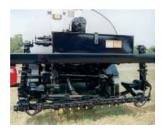
Maintenance distributors offer either an 8' or 10' full circulating spray bar. All bars feature electric-hydraulic gang on/off controls and manual flip valve nozzle control every 4". 10' bars offer 2' folding wings on each side with 1' on each side removable and manual lift and wing fold. Additional 1' add-on sections are also available for either spray bar.
