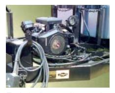
The hydraulic system is powered by an 18 H.P. gasoline engine with electric starter, alternator, battery and 6 gallon fuel tank. The system develops 2500 P.S.I.
