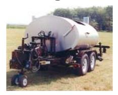
Mounted on a tandem axle, 6" channel frame with electric brakes and safety breakaway, an adjustable pintle eye and crank type jacks front and rear. Two 6000# axles with four LT235/85 R16 (E) tires on disk wheels and flanged steel fenders insure safe, efficient travel. FMVSS-108 lights and wiring and electrical connection for towing vehicle are also provided.
