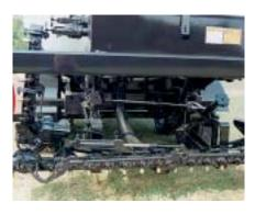
Patented automatic suckback system and coaxial bar feed lines provide complete suckback of the circulating system. Includes all manual valves for loading, circulating in the tank, handspraying and unloading. Pump, valves, and circulating system are manufactured by Etnyre to minimize exposed lines, heat loss and sumps.
