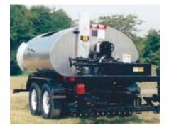
Tank constructed of a 12 gauge steel shell and full section surge plates. Spill collar with 20" manhole with strainers and rollover protection meet HM-198A/HM 183 DOT hot asphalt requirements. Fiberglass 2" insulation covered with aluminum jacketing.
