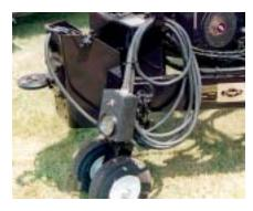
Electric-hydraulic cab control for spray bar gang on-off from the cab is standard equipment with either bar. Spray bar on/off switch is provided in a control panel operated from the towing vehicle cab. The panel is provided with a 20' electrical cord to reach the towing vehicle cab.
